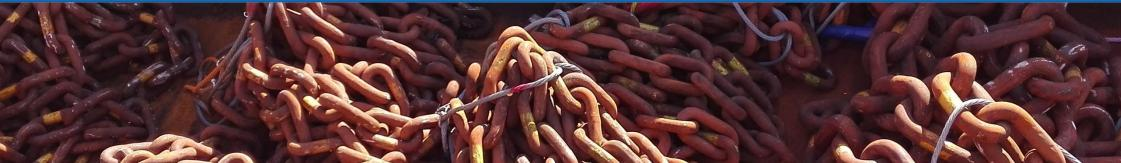
The chain fabrication facility produces chains from 70 mm diameter up to 220 mm diameter in five different steel grades without restrictions in length or weight with an annual capacity of 50.000 tons.
