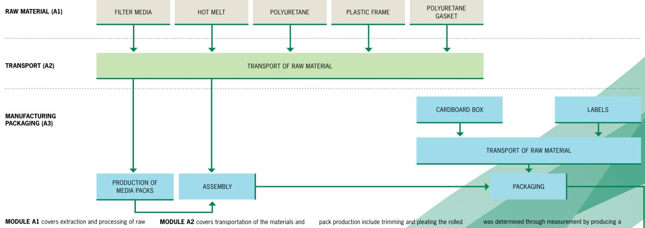
materials, as well as production of the materials and components used for production of Opakfil filters: filter media, plastic frame, hot melt and polyurethane for casting and gasket.
