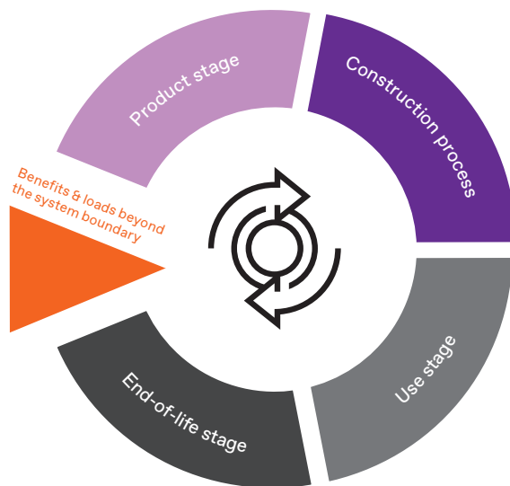
Figure 2: Escalator life cycle stages and respective information modules according to the PCRs
