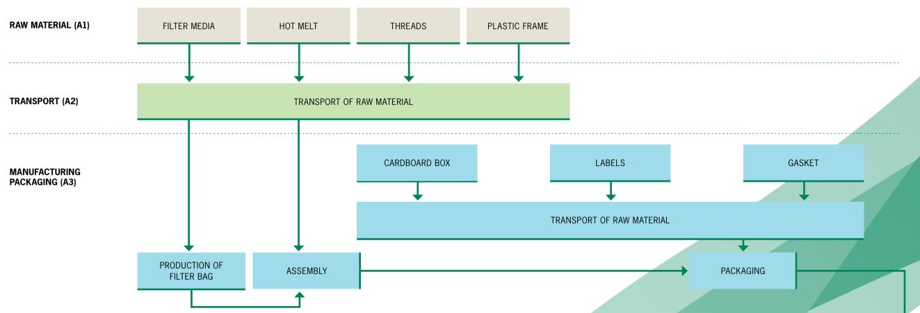
**MODULE A1** covers extraction and processing of raw materials, as well as production of the materials and components used for production of bag filters: filter media, plastic frame, hot melt and threads.
