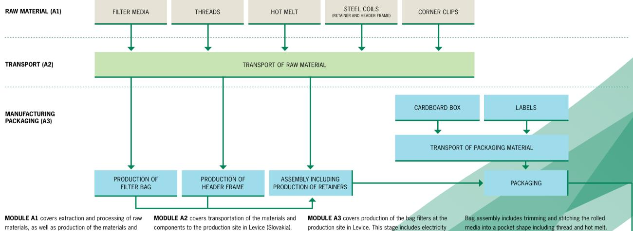
components used for production of bag filters: filter media, steel coils, corner clips, hot melt and threads.
