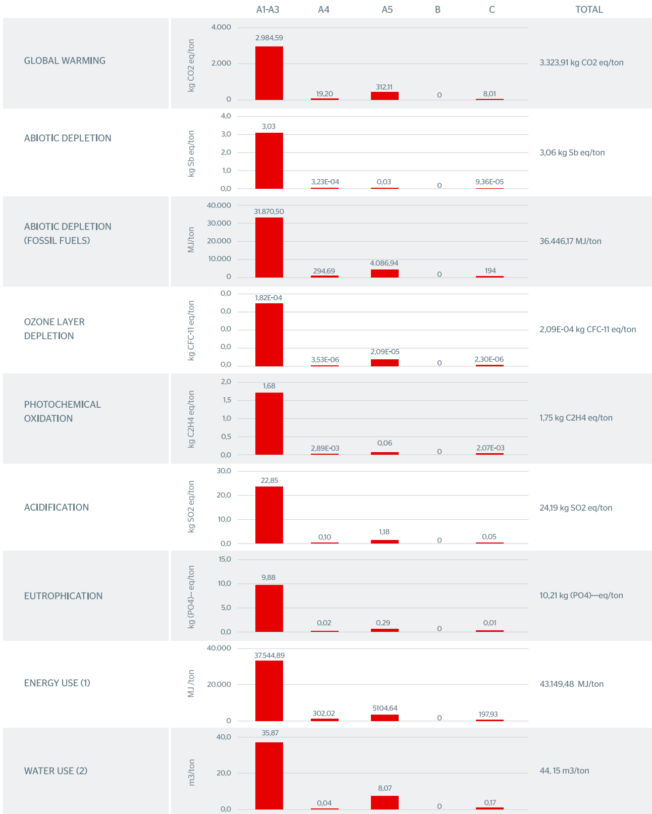
Figure 4 - Interpretation of environmental impact indicators for 1 metric ton of product. (1) Corresponds to total use of primary energy (2) Corresponds to use of net fresh water.
