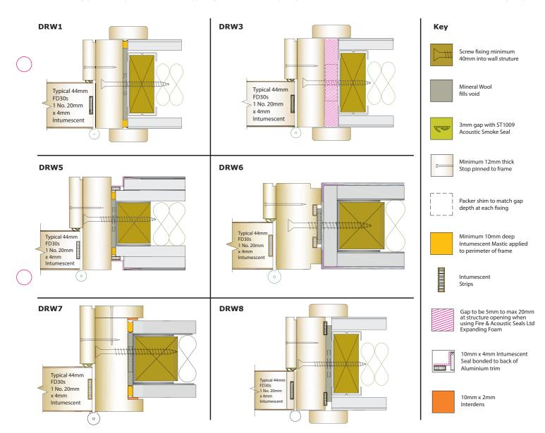
For all other gaps between the frame and the supporting construction (with or without architraves) the method of installation should follow the recommendations of Tables 2 to 5 in BS 8214:2016, "Timber based fire door assemblies - Code of Practice", using fire seal products proven in linear timber applications.
