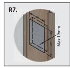
R7. Leaf face recess re-instated Maximum size timber (640kg/m3) face plate infill: 200mm high x 100mm wide x 19mm deep.
