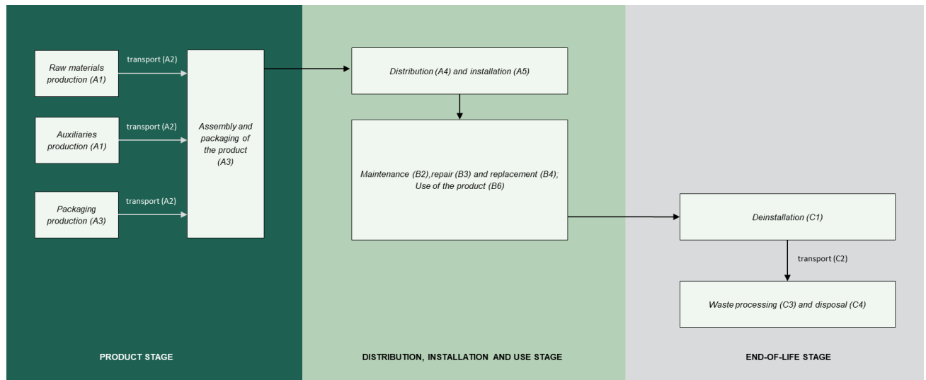
Figure 2. Process flow diagram illustrating the processes that shall be included in the product system, divided into the life-cycle stages. The illustration of processes to include may not be exhaustive.
